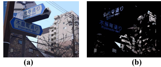
Figure 4. Effect of cascade classifier: (a) input clustered image, (b) result of cascade classifier
